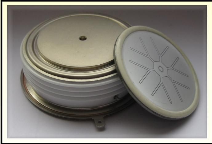
IXYS UK Westcode Ltd. announces a new pressure contact distributed gate thyristor with increased power density. This new fast thyristor with turn-off time of as little as 20 $\mu$ s and current rating 1955A, is symmetrical blocking with  $V_{drm}/V_{rrm}$  equal to 1600V and therefore suitable for both voltage and current fed applications.
